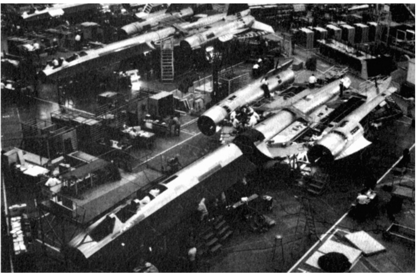
Blackbird production line at the Skunk Works. In mid-1970s, they produced a new Blackbird every month. ( Lockheed )
